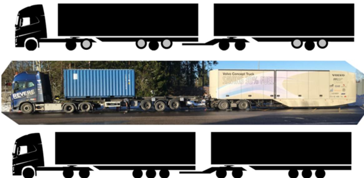
Figure 7 **Top and Bottom** the schematic combination with lifted and non-lifted axels. **Middle** the vehicle combination used in the Coast Down test. Note that five axels are lifted on the photo in the middle; one on the tractor, two on the first semitrailer and two on the second semitrailer (not seen on the second semitrailer due to side covers). The vehicle was used for measurements with all axels down as well as with lifted axels.
