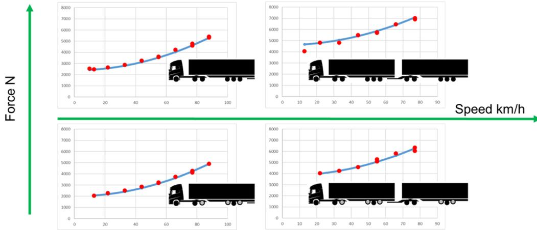
Figure 10 Comparison of measurements (red) and the numeric solution (blue) Constant Speed tests
