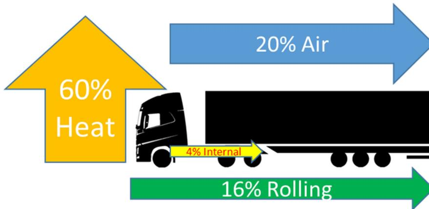
Figure 1 Schematic power use at 80 km/h on flat road
