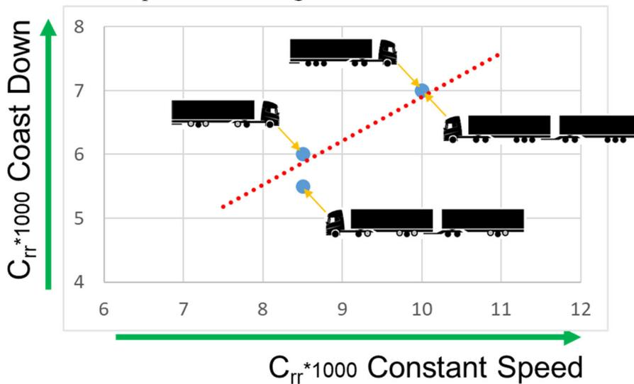
Figure 9 Correlation between Rolling Resistance coefficient ( $C_{rr} * 1000$ ) estimations from the Constant Speed and Coast Down Tests. Blue circle estimations of  $C_{rr}$  using the two methods. Red line shows correlation between the  $C_{rr}$  estimations for the single and duo trailers.
