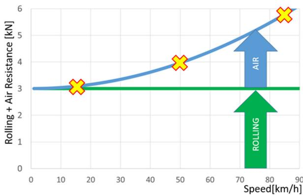
Figure 4 Schematic diagram of measured total resistance (rolling + air). Yellow and red cross (X) are examples of measurements at various speeds (15, 50 and 85 km/h).
