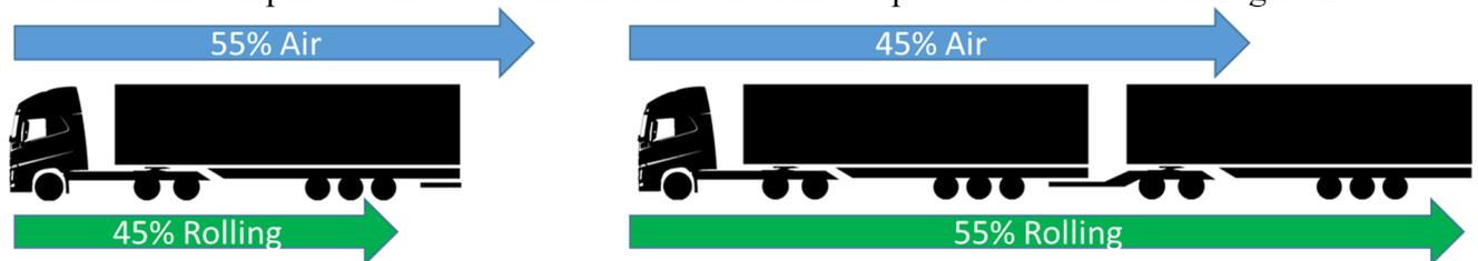
Figure 2 Relative power use between Air drag and Rolling Resistance for single and duo trailer combinations at 80 km/h
