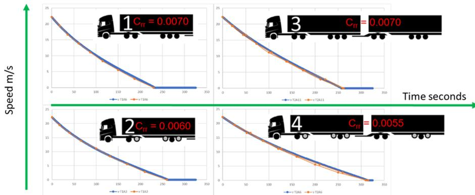
Figure 11 Comparison of measurements (red) and the numeric solution (blue) for Coast Down test
