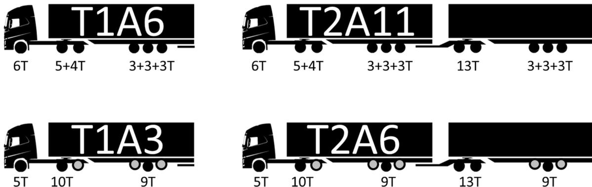
Figure 5 The four vehicle combinations in the tests. The letter T stands for trailers and A for axles. T1A3 indicates three axles used on the combination with one semitrailer.
