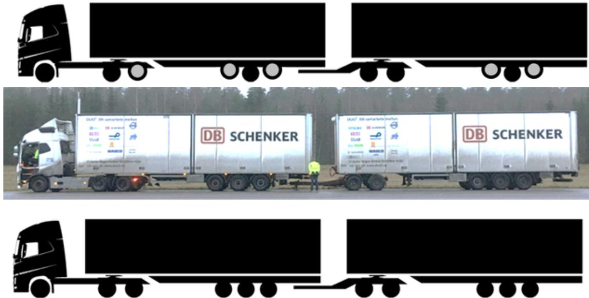
Figure 6 **Top and Bottom** the schematic combination with lifted and non-lifted axels. **Middle** the vehicle combination used in the Constant Speed test. Note that the axels are not lifted on the photo in the middle. The vehicle was used for measurements with all axels down as well as with five lifted axels.
