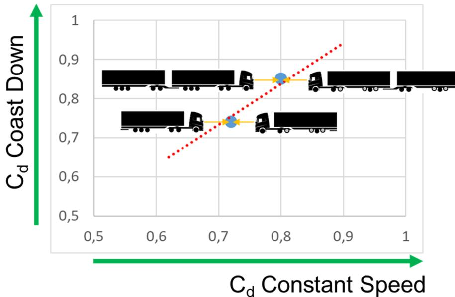
Figure 8 Correlation between Air drag coefficient ( $C_d$ ) estimations from the Constant Speed and Coast Down Tests. Blue circle estimations of  $C_d$  using the two methods. Red line shows correlation between the  $C_d$  estimations for the single and duo trailers.
