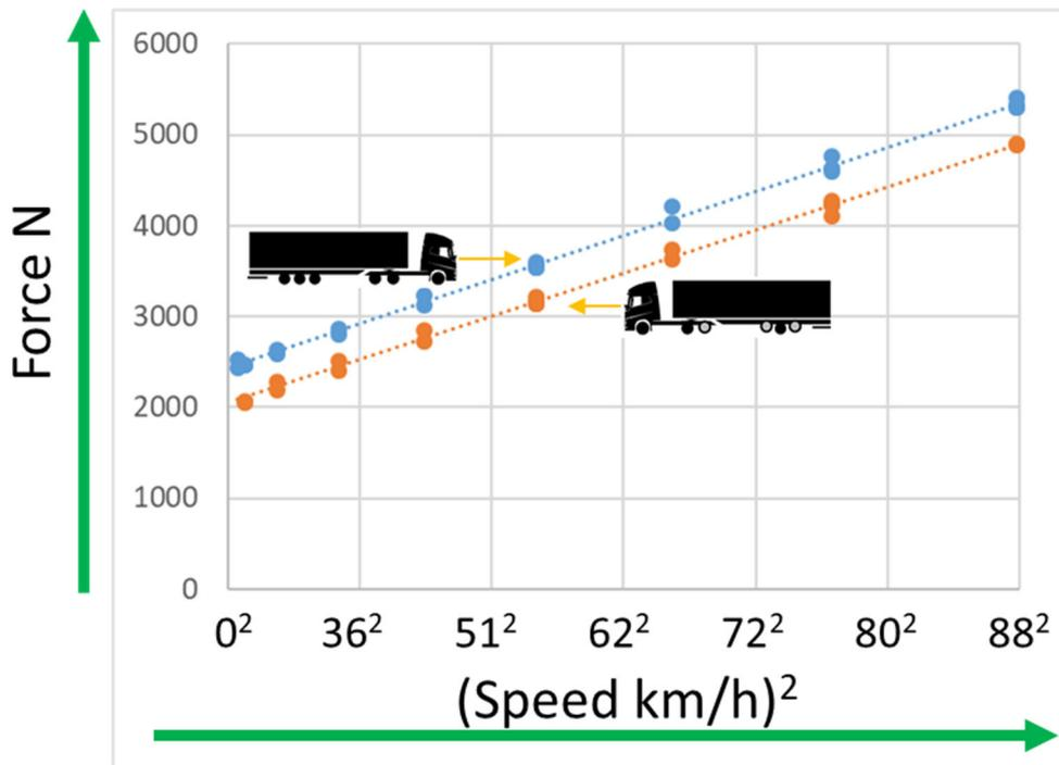
Figure 12 X-axis: Speed to the power of two. Y-axis: is the combined air and roll resistance. Force measured during Constant Speed test. Blue, all axels down, and Red 3 of 6 axels lifted. Dotted lines are linear fit in accordance with European test method<sup>4</sup> for air resitance. The two lines are parallel which means that the air resistance is the same for both cases.
