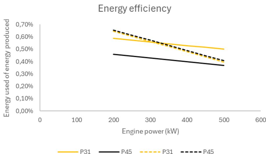
Figure 3. Energy efficiency (the energy used by the chipper in relation to the energy in the chips produced) when chipping stemwood (solid lines) and logging residues (dashed line) with a moisture content of 40% into P31 or P45 size chips using a drum chipper where the engine powers the chipper, loader and base machine.
