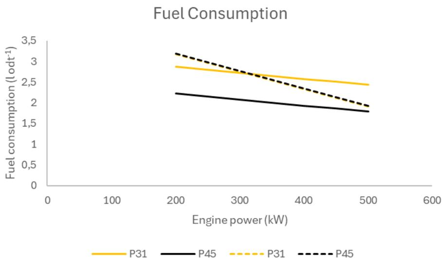
Figure 2. Fuel consumption when chipping stemwood (solid lines) and logging residues (dashed line) with a moisture content of 40% into P31 or P45 size chips using a drum chipper where the engine powers the chipper, loader and base machine.
