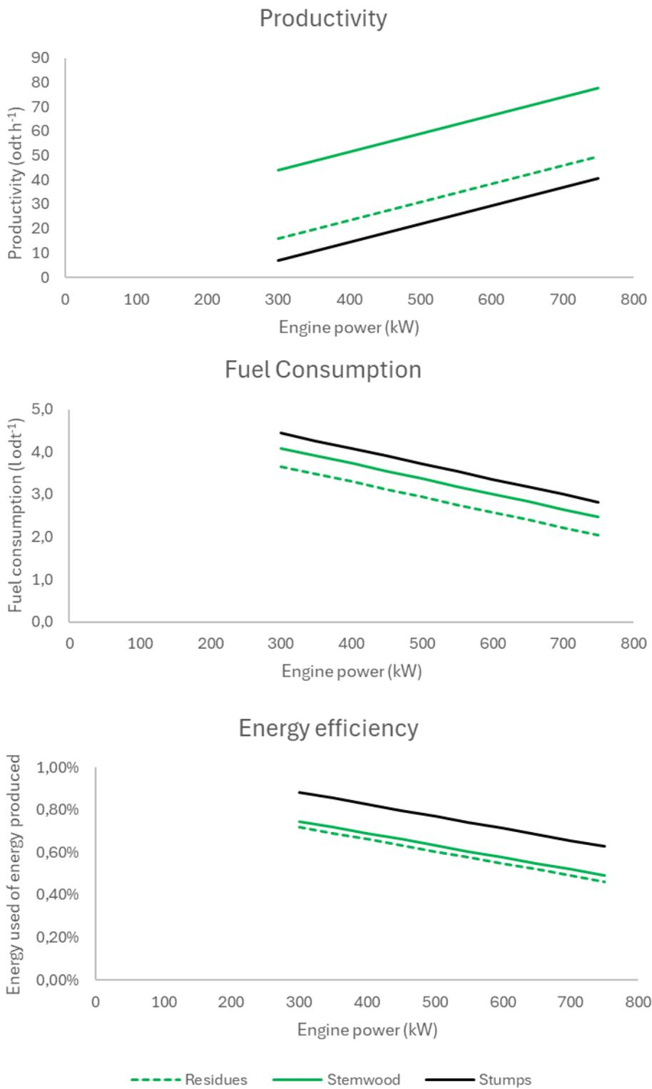
Figure 4. Productivity (odt h<sup>-1</sup>), fuel consumption (l odt<sup>-1</sup>) and energy efficiency (J J<sup>-1</sup>) for hammermills producing chips (hog fuel) from stemwood, logging residues, and stumps. Note that the engine usually is not powering the loader feeding the hammermill.
