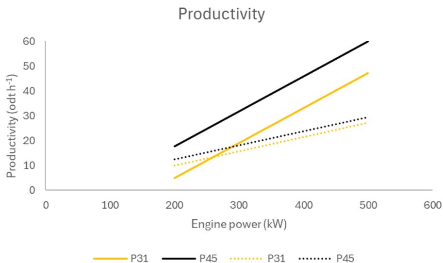
Figure 1. Productivity when chipping stemwood (solid lines) and logging residues (dashed line) into P31 or P45 size chips using a drum chipper where the engine powers the chipper, loader and base machine.
