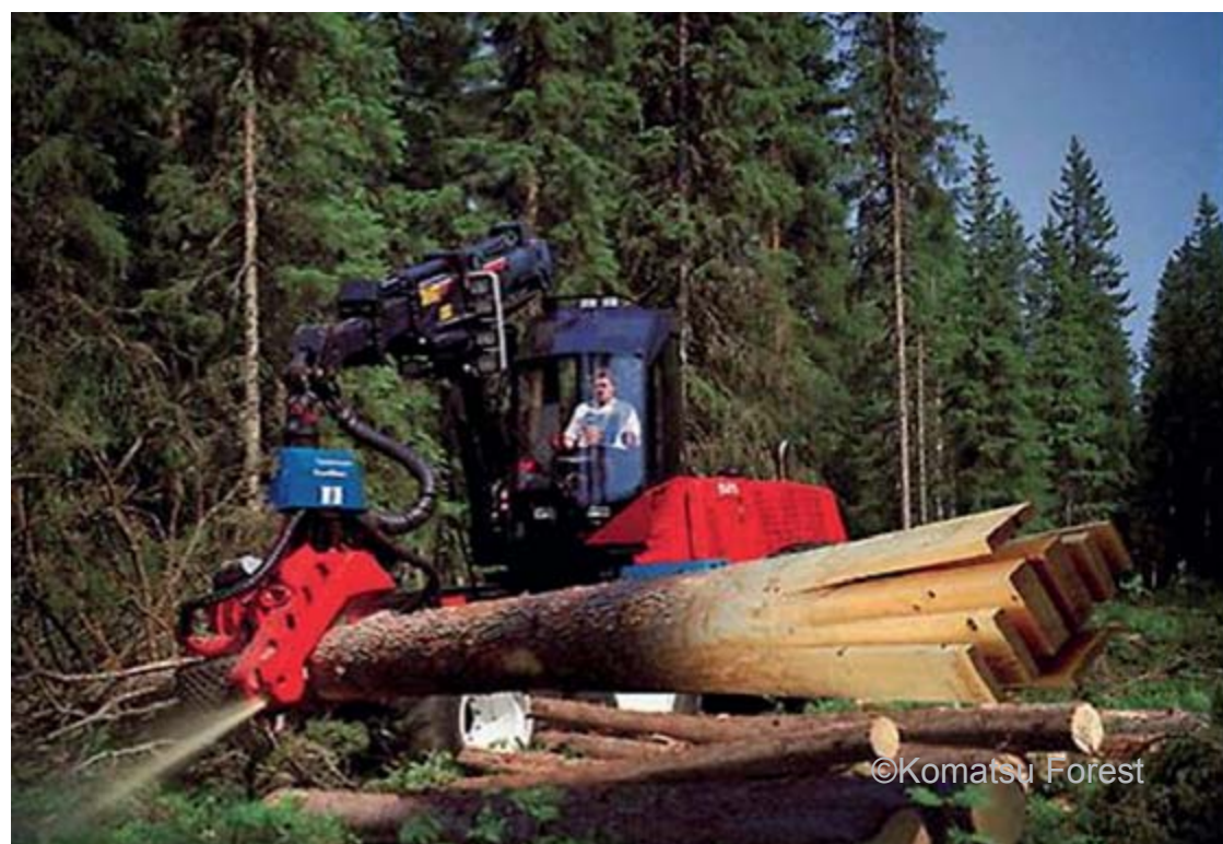
Figure 14. Manufacturing starts in the forest. In CTL(Cut To Length) systems the selection, bucking alternatives and sorting of produced wood are all decided at harvesting (Photo Komatsu Forest)
