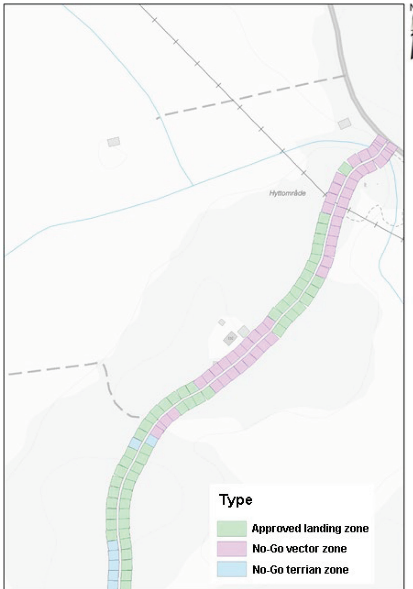
Figure 4. The colour codes show the classification given to each road zone after analysis with the obstacles. In the middle of the map, for example, a residential plot can be seen that generates a No-Go vector zone, and similar No-Go zones were generated near an ancient monument and a road junction in the north. In the southern part of the map, individual No-Go terrain zones can be seen where the requirement for a maximum height deviation of two metres was not satisfied.
