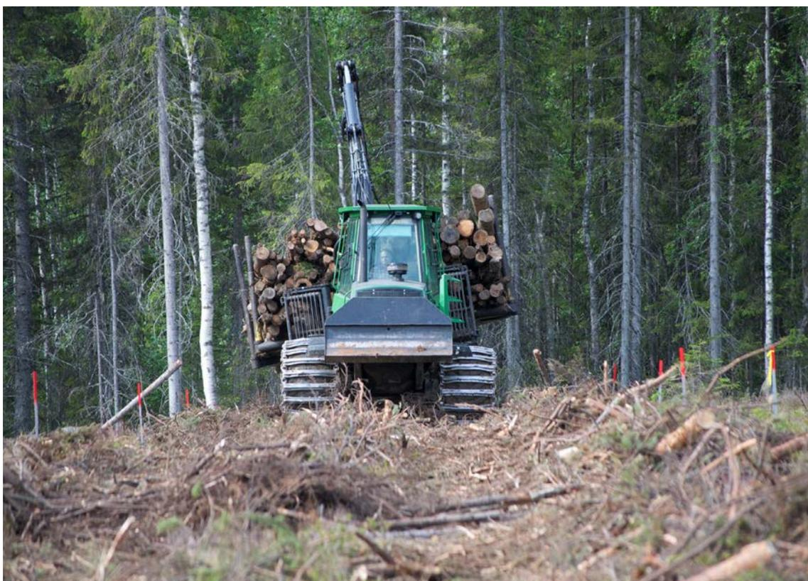
The forwarder driving uphill at the Trågalidsberget site on a study plot with logging residue for ground protection. Photo Eva Ring
