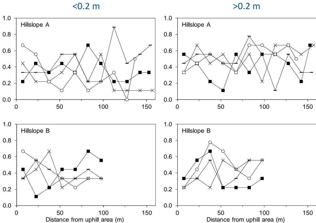
Fig. 15. Proportion of metal probe insertions <0.2 m (left) or >0.2 m (right) on the 15 m × 15 m subplots (in total 9 insertions per subplot) for the study plots at Rotflakamyran hillslope A (above) and B (below). The distance from the upslope short side refers to the centre of each subplot. ○: Ctrl, ■: No protection, ×: Logging residue, -: Logging mats.
