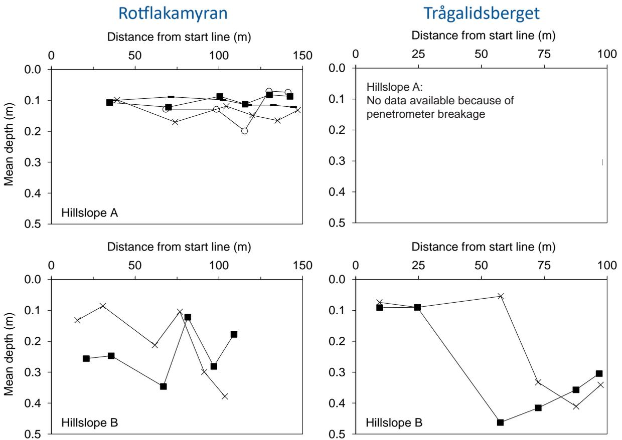
Fig. 17. The mean maximum cone penetration depth at Rotflakamyran (left) and Trågalidsberget (right) before treatment. Six measurements per transect were performed along T1-T6 at Rotflakamyran hillslope A and 12 measurements per transect for hillslope B at both sites. ○: Ctrl, ■: No protection, ×: Logging residue, -: Logging mats
