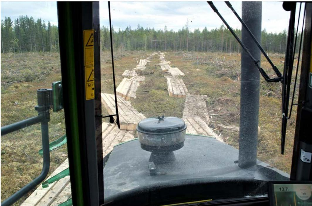
Fig. 20. Rotflakamyran hillslope A. Above: Placement of logging mats from the forwarder wood bunk using the boom-mounted grip. Below: Driving on the mats – view from the forwarder cabin. Photo Eva Ring
