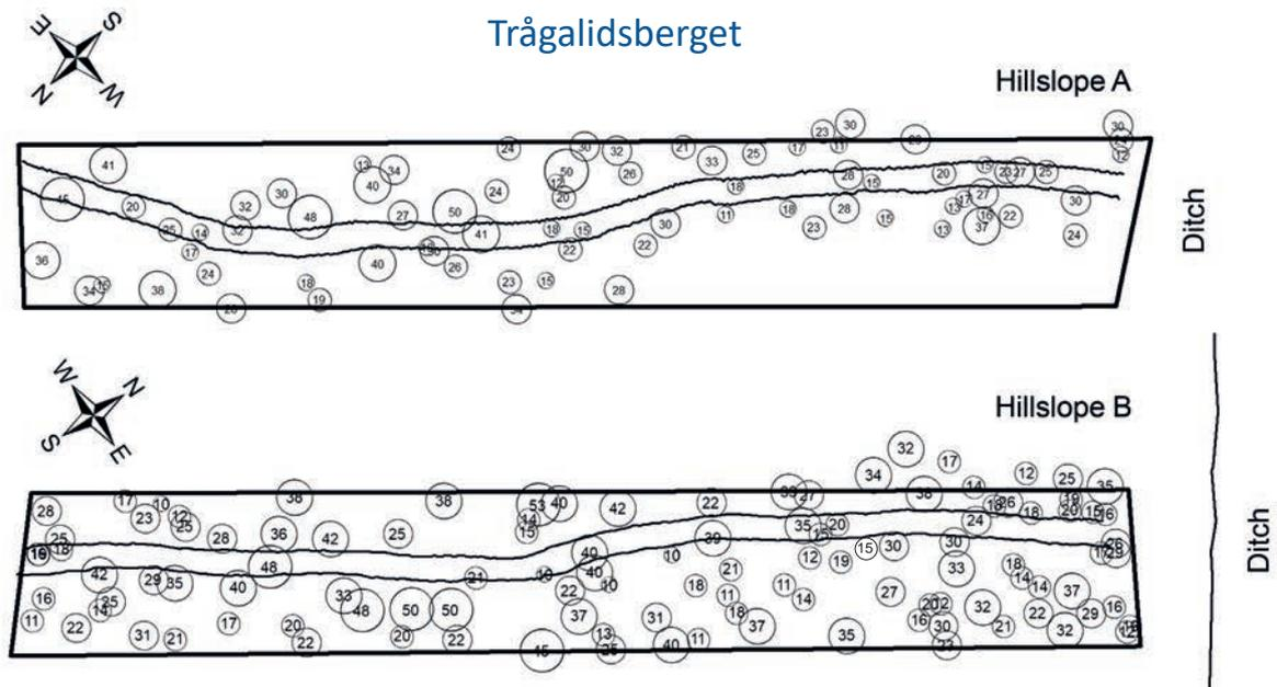
Fig. 12. Locations and diameters of stumps, with a diameter greater than 10 cm, on the study plots without ground protection (NoProt) at Trågalidsberget hillslopes A (adjacent to the wheel tracks) and B. The start line is to the left. The solid lines on the study plots show the forwarder's wheel tracks.
