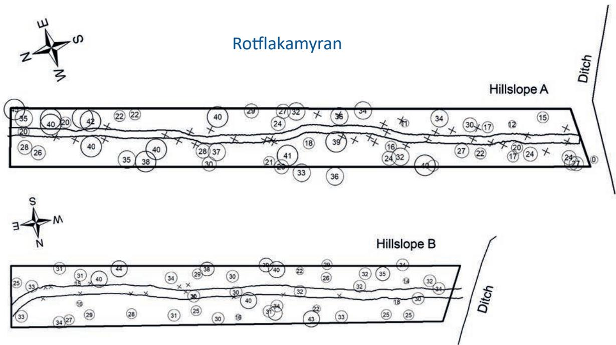
Fig. 11. Locations and diameters of stumps, with a diameter greater than 10 cm, on the study plots without ground protection at Rotflakamyran hillslopes A and B. The start line is to the left. "x" indicates stumps without diameter measurements. The solid lines on the study plots show the forwarder's wheel tracks.
