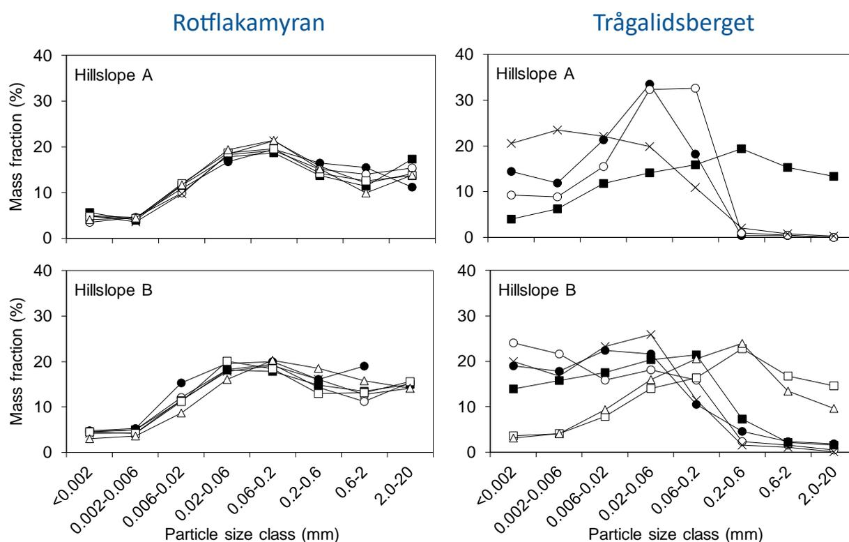
Fig. 13. Mass fraction of eight particle size classes in the mineral soil at 0 to 20 cm depth at Rotflakamyran and Trågalidsberget. The analysed soil samples were collected in the control plots along transects 1-6 (T1-T6). At Trågalidsberget hillslope A, a large number of stones prevented sampling of transects 1 and 2.  $\Delta$ : T1,  $\square$ : T2;  $\blacksquare$ : T3,  $\times$ : T4,  $\circ$ : T5,  $\bullet$ : T6.
