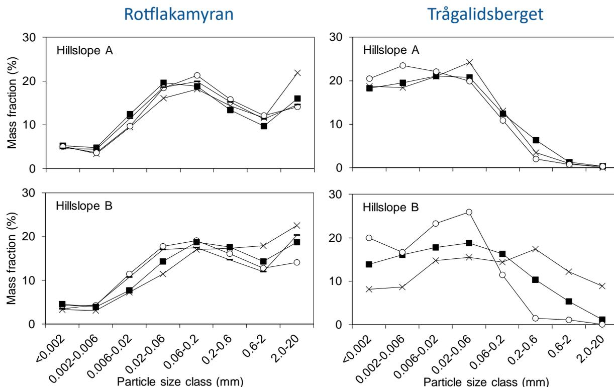
Fig. 14. Mass fractions of eight particle size classes for the mineral soil at 0 to 20 cm depth for transect 4 (T4) at Rotflakamyran (left panel) and Trågalidsberget (right panel). ○: Ctrl, ■: No protection, ×: Logging residue, - : Logging mats.
