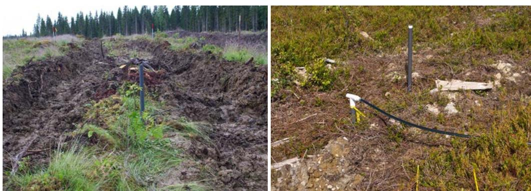
Fig. 24. Left: A groundwater tube in the study plot with no ground protection at Trågalidsberget hillslope B (in the downhill area). Right: A groundwater tube with a CS450 pressure transducer mounted using an open/ventilated T-coupling (lower left) and a tube used for groundwater sampling (with the longest aboveground tube length). Photo Eva Ring
