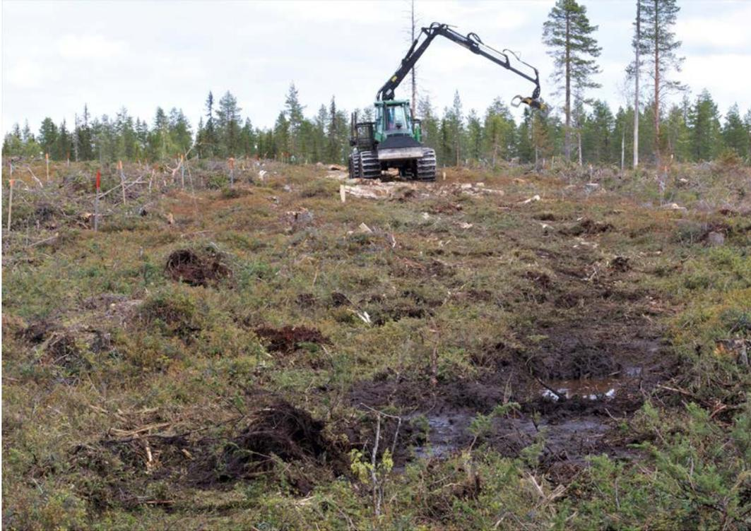
Fig. 27. Rutting in the study plot with logging mats at Rotflakamyran hillslope A, caused by the forwarder slipping off the mat. The photo also shows the forwarder when removing the mats after driving, starting downhill and moving uphill. Photo Eva Ring
