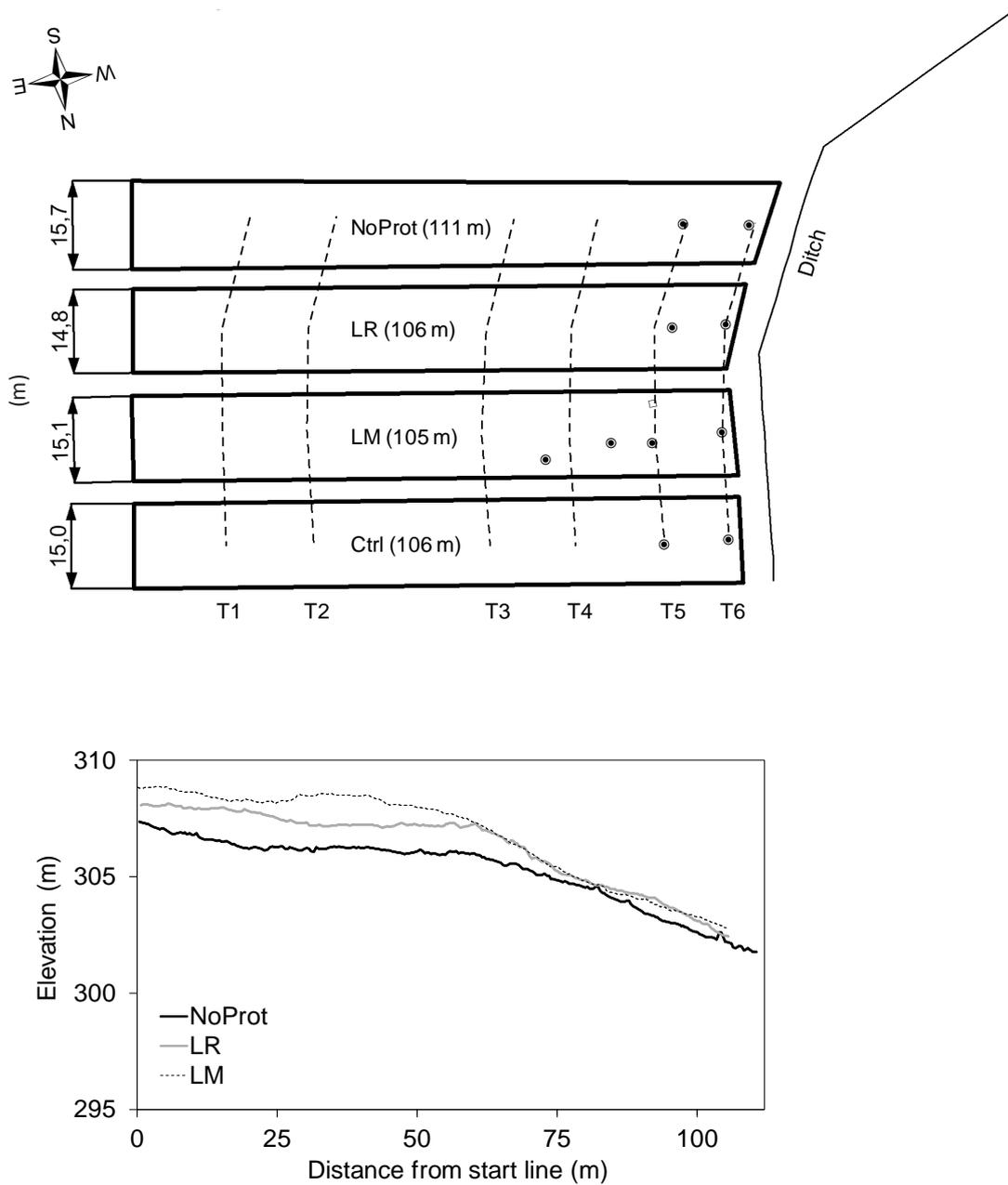
Fig. 5. Top: Size (in metres) of the study plots, and location of groundwater tubes (●), logger (□) and transects T1-T6 at Rotflakamyran hillslope B. Bottom: Hillslope profiles of the study plots subjected to driving (note the different scales on the x- and y-axes, exaggerating inclination). The profiles show the interpolated original soil surface above the right rut, using GNSS-positioning and Triangular Irregular Networks. NoProt: No ground protection, LR: Logging residue, LM: Logging mats.
