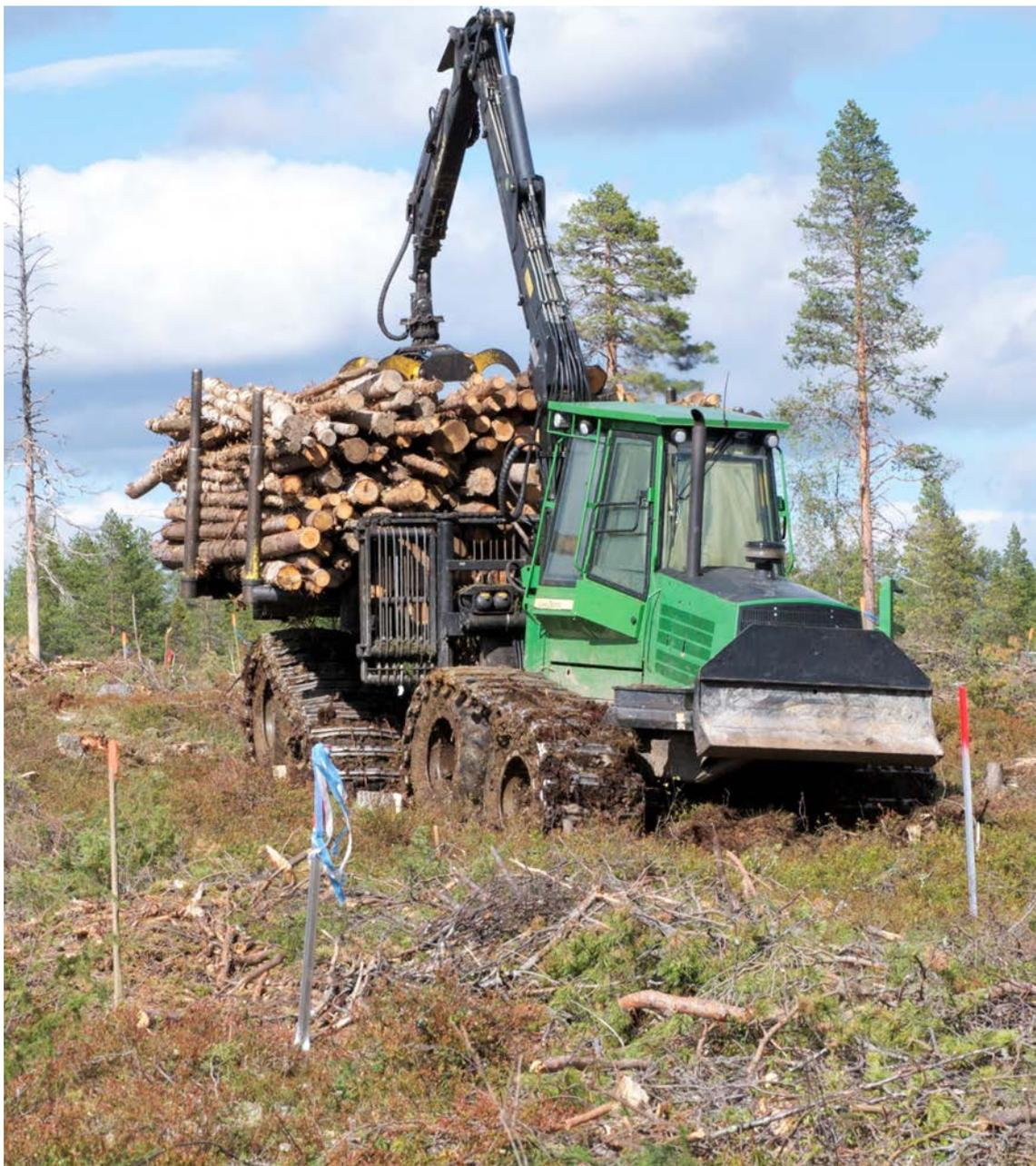
Fig. 18. The treatments were performed using a John Deere 1410D forwarder with eight wheels and 710 mm wide tires with a tire pressure of 350 kPa and 500 kPa for the tractor and wood bunk, respectively. Bogie tracks were mounted both on front (Olofsfors ECO-TRACKS) and rear (Clark Terra Lite) wheel pairs. The forwarder was operated by the same driver at both sites. Photo Eva Ring
