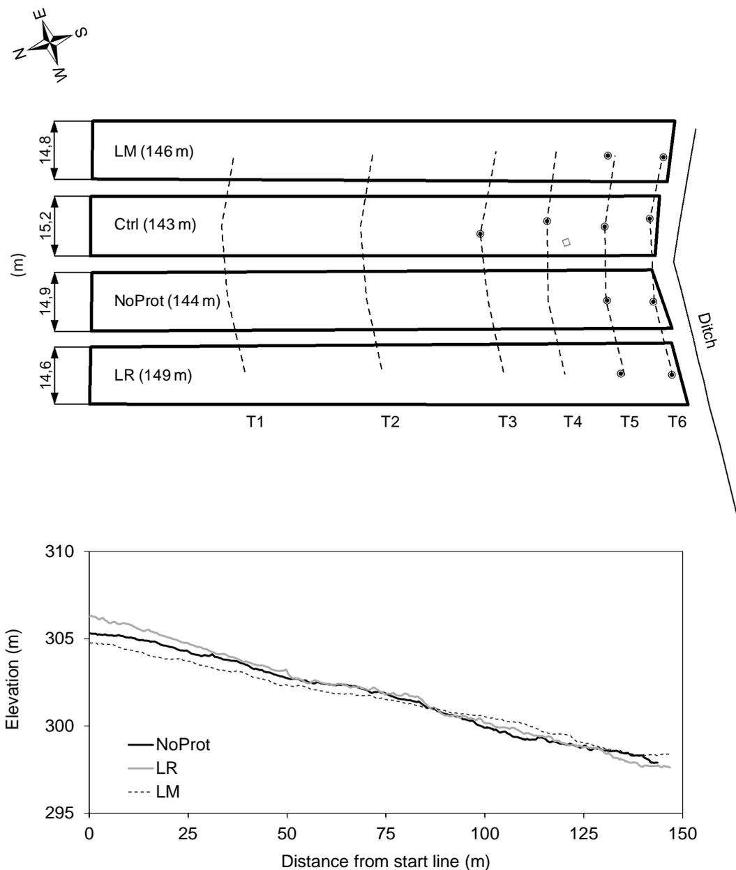
Fig. 4. Top: Size (in metres) of the study plots, and location of groundwater tubes (●), logger (□) and transects T1-T6 at Rotflakamyran hillslope A. Bottom: Hillslope profiles of the study plots subjected to driving (note the different scales on the x- and y-axes, exaggerating inclination). The profiles show the interpolated original soil surface above the right rut, using GNSS-positioning and Triangular Irregular Networks. NoProt: No ground protection, LR: Logging residue, LM: Logging mats.
