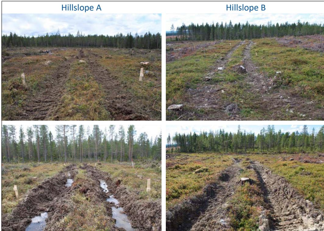
Fig. 25. Rutting on the study plots subjected to forwarder traffic with no ground protection at Rotflakamyran one day (hillslope A) and two months (hillslope B) after treatment. Above: Rutting in the upper part of the hillslopes (defined as “0 cm” when measured manually). Below: Rutting in the lower parts—all views are downhill. Photo Eva Ring
