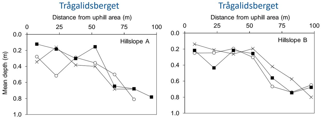
Fig. 16. Metal probe insertion depth along the study plots at Trågalidsberget (mean depth per subplot). The depths presented for the most downhill area (lower 30-45 m) of hillslope B are underestimated because a definite depth could not be determined in many cases. ○: Ctrl, ■: No protection, ×: Logging residue.
