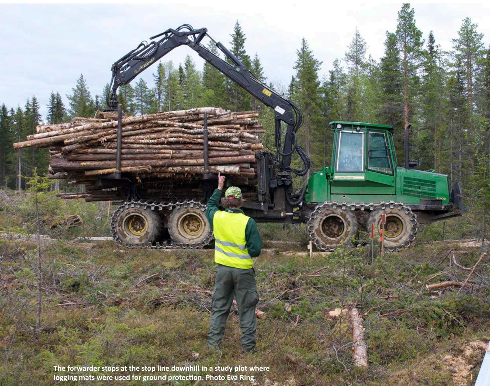
The forwarder stops at the stop line downhill in a study plot where logging mats were used for ground protection. Photo Eva Ring
