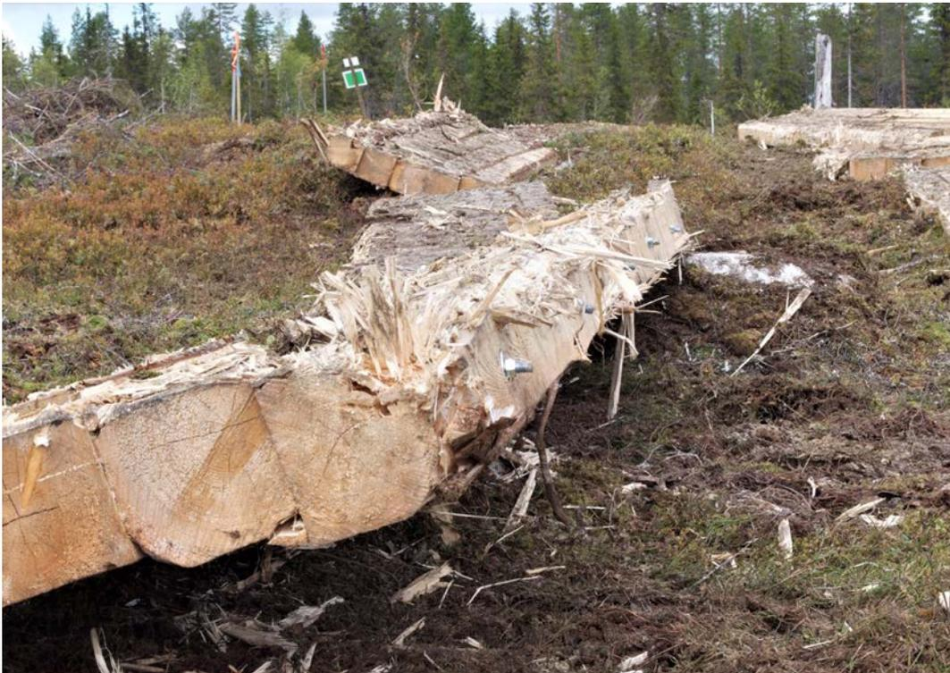
Fig. 28. Driving on logging mats applied on uneven ground resulted in significant wear of the mats. Photo Eva Ring
