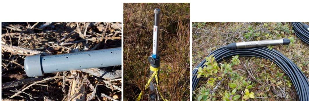
Fig. 23. Equipment used for monitoring the groundwater level: a groundwater tube with bottom cap (left), a 1-m long water height probe (TruTrack WT-HR 1000) installed in a groundwater tube (centre), and a pressure transducer (Campbell CS450) (right). Photo Eva Ring
