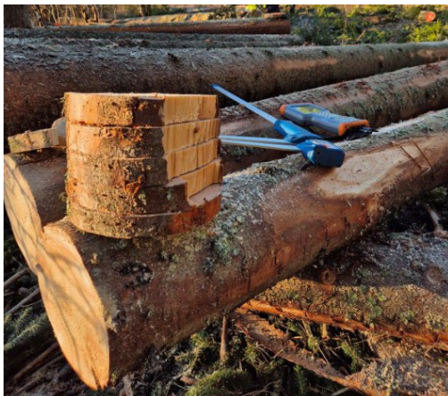
Figure 27. The disc method of measuring bucking splits. The wood discs are cut from the same log end, and the length of the bucking split can be estimated by summing the thickness of the discs. Photo: Björn Hannrup, Skogforsk.
