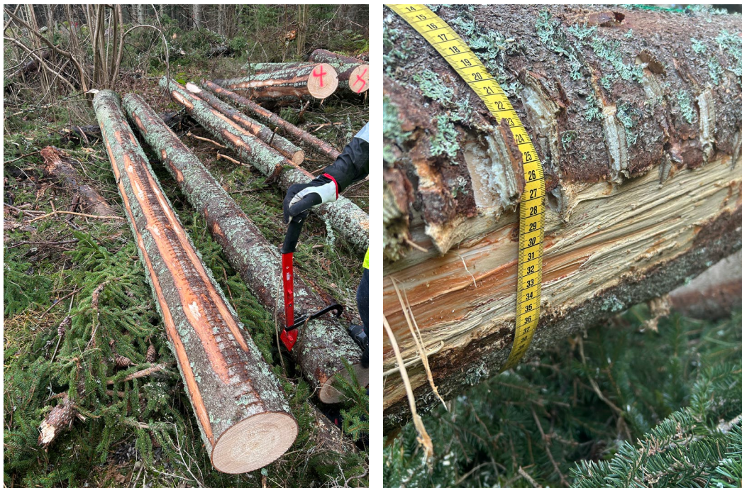
Figure 39. Two images illustrate three types of bark damage. The left image shows a high level of bark damage caused by the delimbing knives, however most of the inner bark remains intact. The right image shows two types of damage side by side. The completely peeled section illustrates bark damage that has exposed wood. The cuts above it shows feed roller penetration that has also exposed wood. This type of feed roller damage was observed only on Eco Log stems. Although the feed roller penetration appears severe in the image, most penetration depths were no greater than 7 mm. For further details, see previous section on feed roller spike damage.
