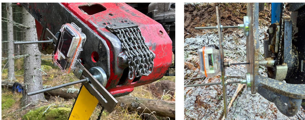
Figure 18. Rotary encoder connected to the sprocket hub for measuring the saw motor speed. The pulses and their timestamps were logged locally and streamed via Bluetooth to a mobile phone, which also controlled the start and stop times for data collection. Photo: Björn Hannrup, Skogforsk.
