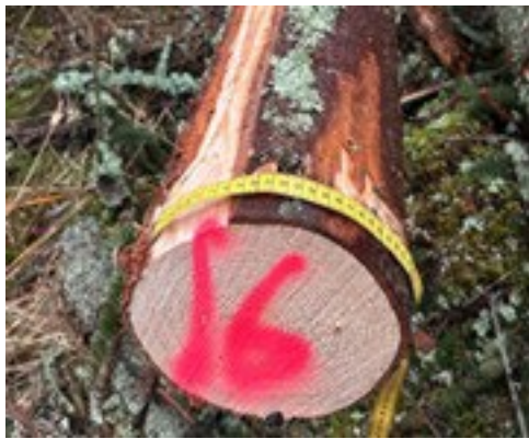
Figure 29. Illustration of the definition of bark stripping and how it was measured in practice. Bark stripping was assessed in two classes: exposed wood and inner bark remaining.
