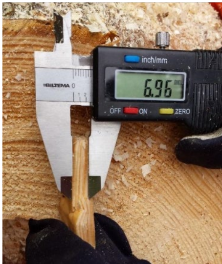
Figure 3. The feed roller spike damage was measured with callipers.
