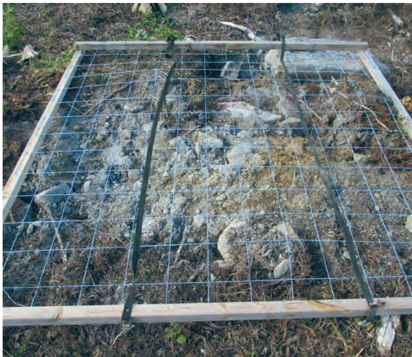
Measurement of the affected ground around a stump cavity left by the TL-GROT stump head. Each square is 15 x 15 cm.
