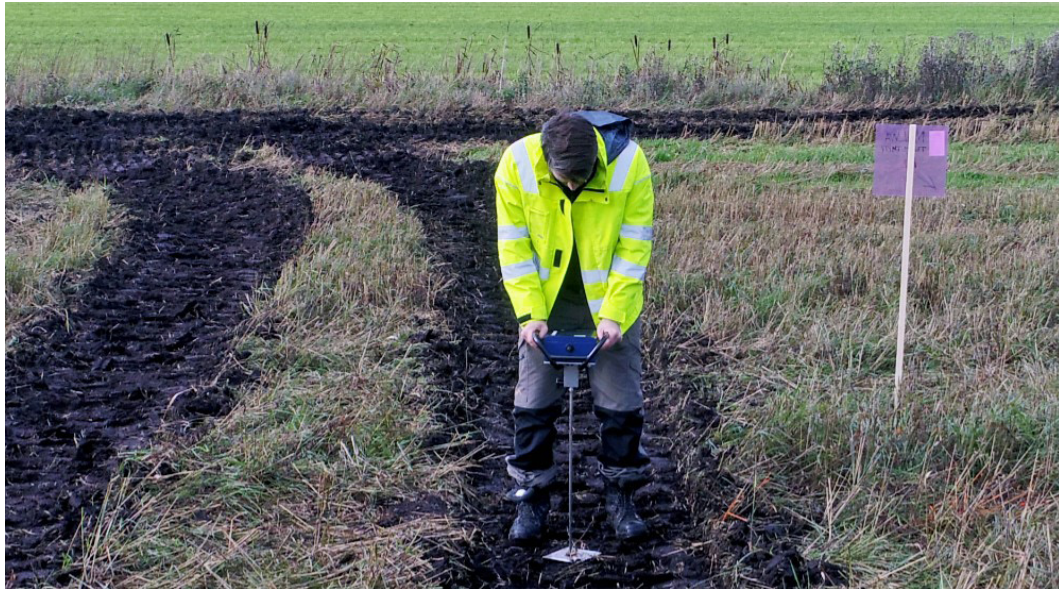
Figure 14. Cone penetration resistance was measured before, in middle of and after completion of each rutting test. Foto: Rolf Björheden, Skogforsk.
