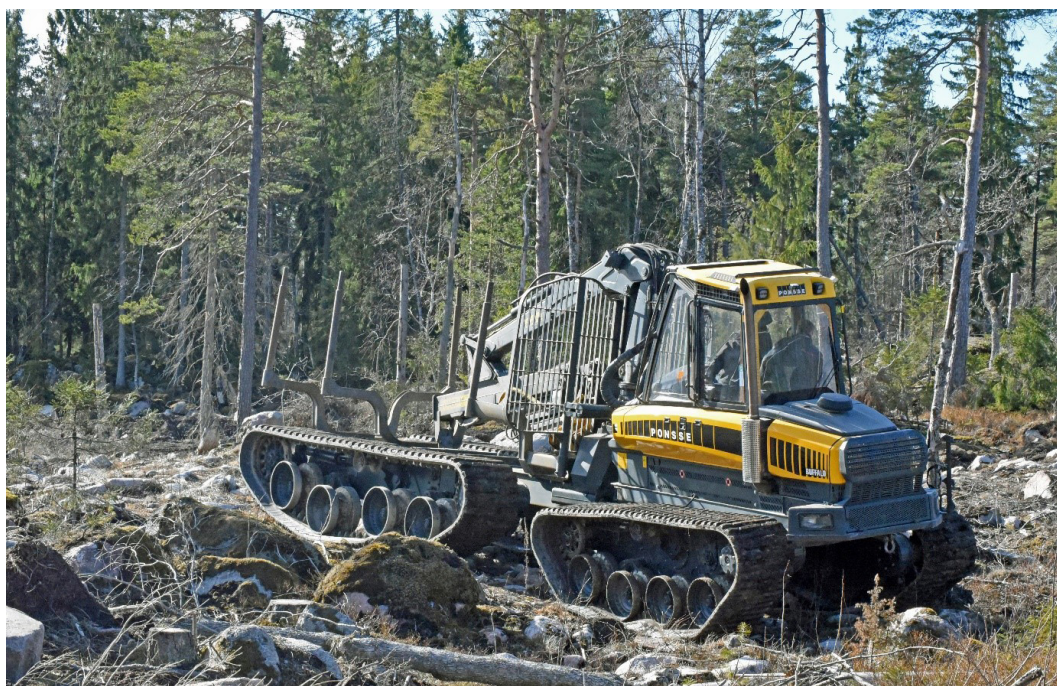
Figure 27. Surface roughness trafficability test in Jälla, Sweden. The OnTrack configuration with a fixed long rear track unit showed favourably low vibration levels. Foto: Rolf Björheden, Skogforsk.
