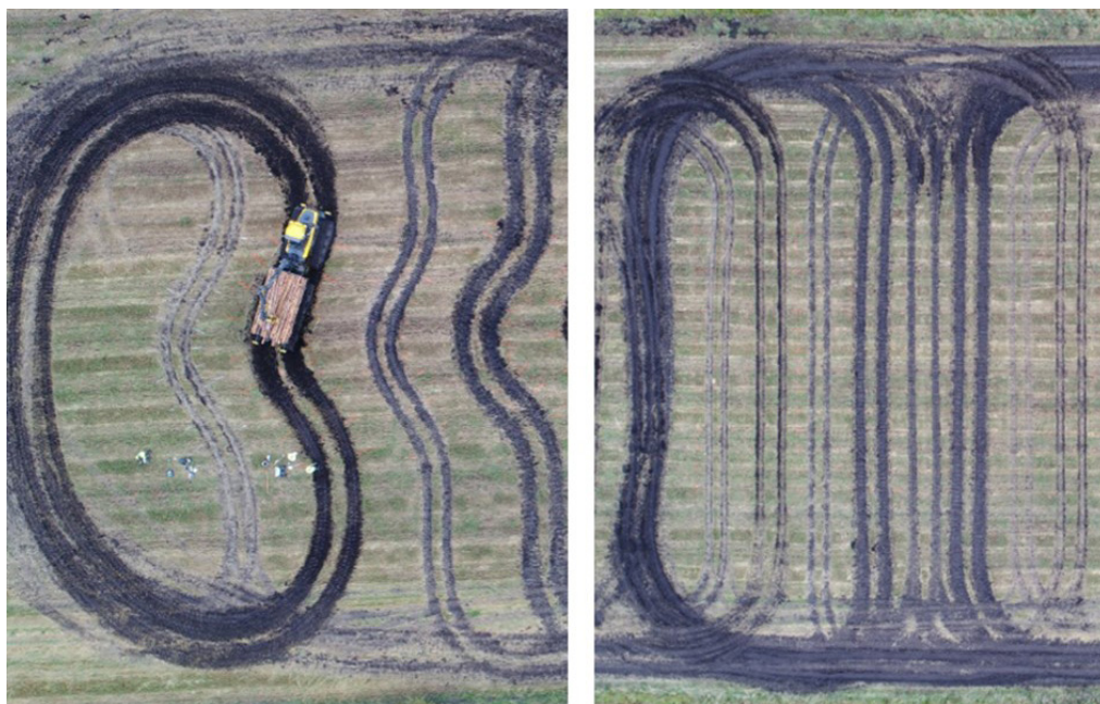
Figure 11. Aerial view showing the layout of the 'slalom' (left) and straight (right) rut formation test tracks.
