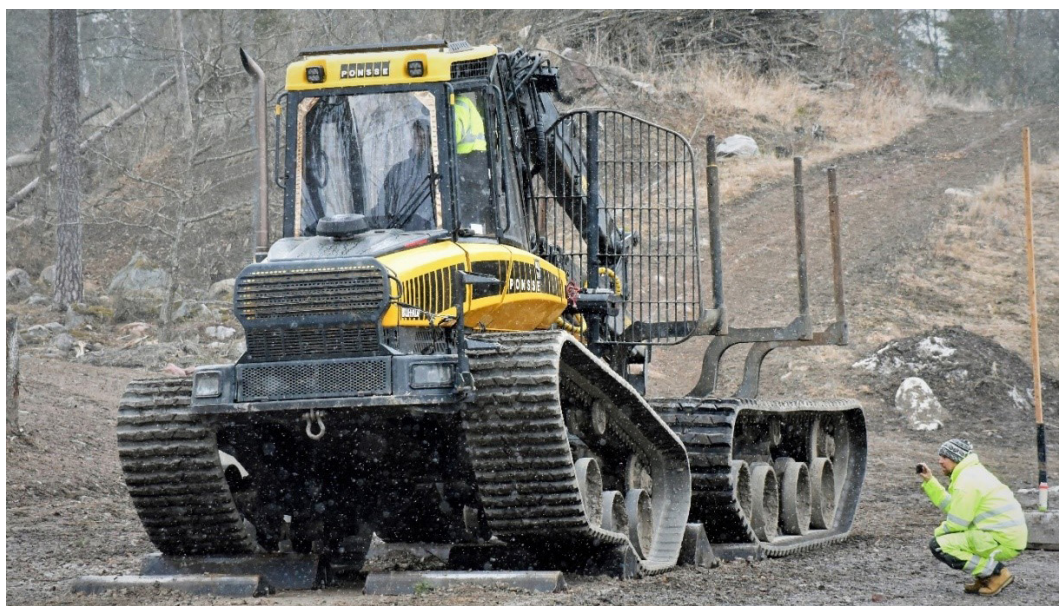
Figure 16. Standardized measurement of the operator's exposure to whole-body vibrations for the initial OnTrack configuration, OnTrack PF, were performed in March 2017 in Jälla, Sweden.
