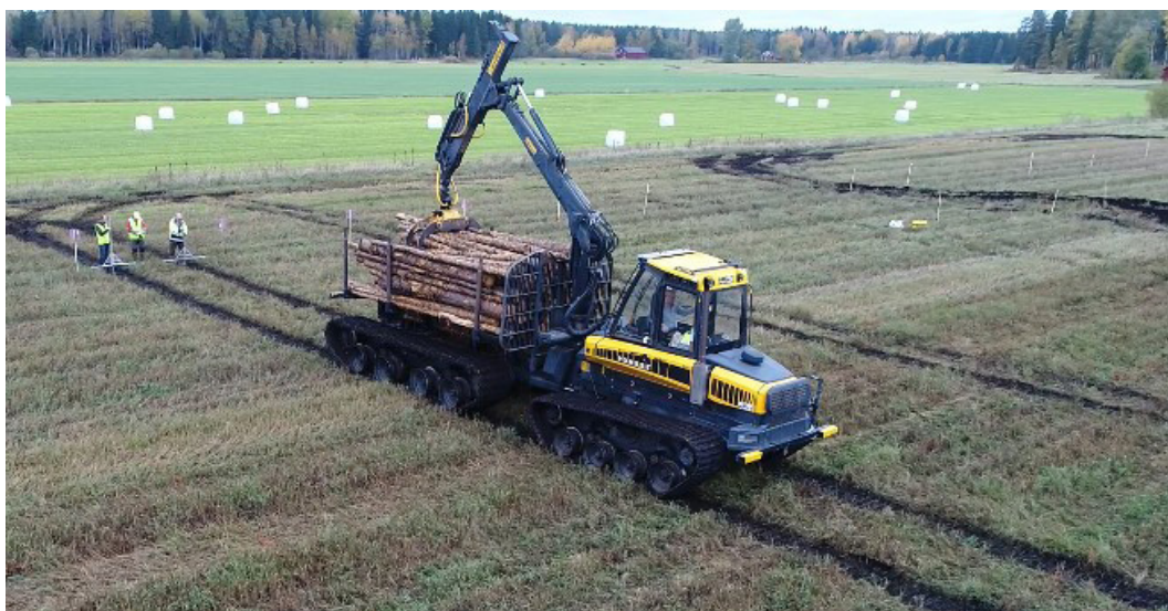
Figure 9. The laden OnTrack during the rut formation tests. Foto: Rolf Björheden, Skogforsk.
