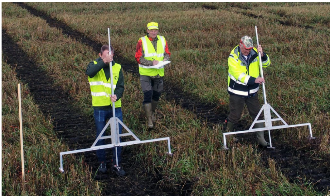
Figure 12. Rut depth measurement on the straight rutting test tracks. Foto: Bruce Talbot, Nibio.
