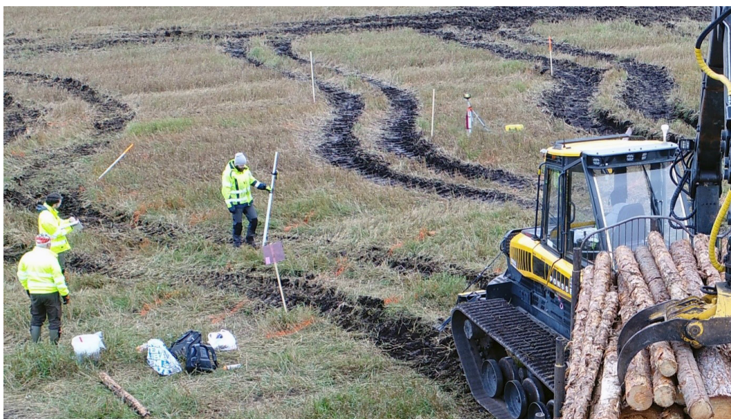
Figure 13. Rut depth measurement with rotating laser and measuring stick on the 'slalom' rutting test tracks. Foto: Rolf Björheden, Skogforsk.
