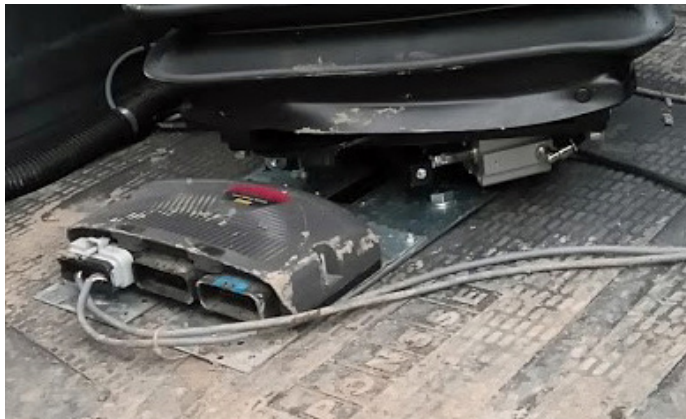
Figure 3. IMU installed above the front bogie axle under the driver's seat. Foto: Rolf Björheden, Skogforsk.
