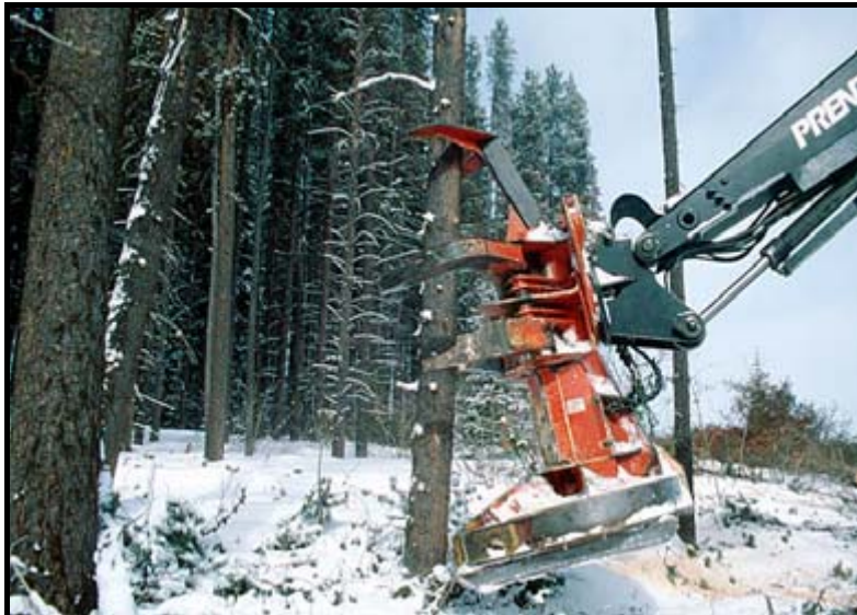
Figure 8. Bending forces applied to tree during felling.
