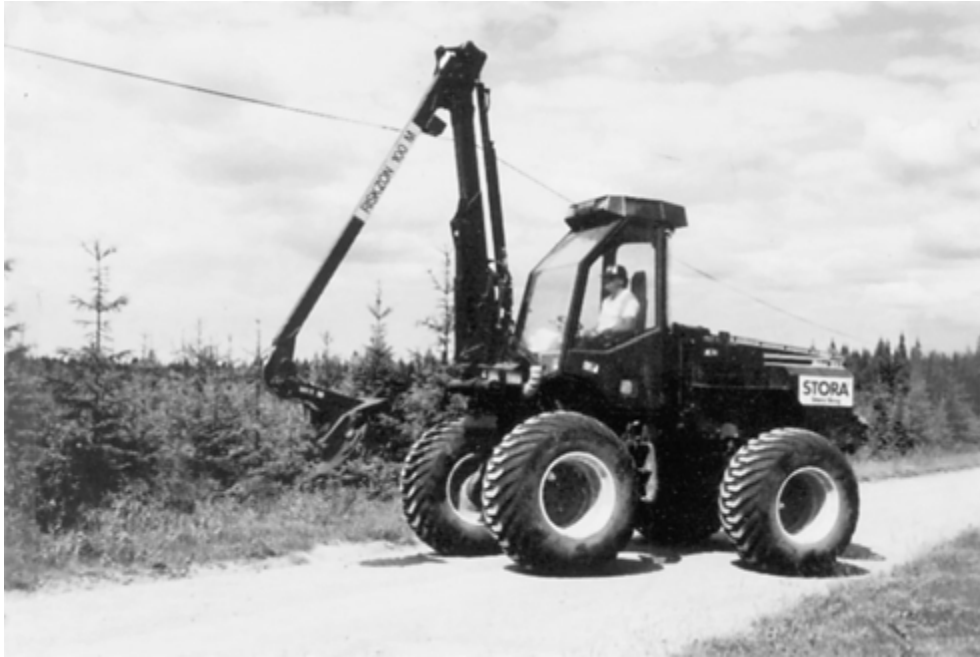
Fig. 2. The Lillebror 504 R cleaning machine. It weighs 5.5 tonnes, has a ground clearance of 90 cm and, as pictured here, is equipped with an MKR-80 cleaning head.
