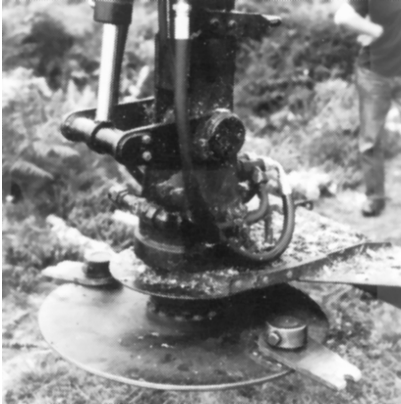
Fig. 3. The Häglinge cleaning head, comprising a steel disc 80 cm in diameter and two pivot-mounted flails.
