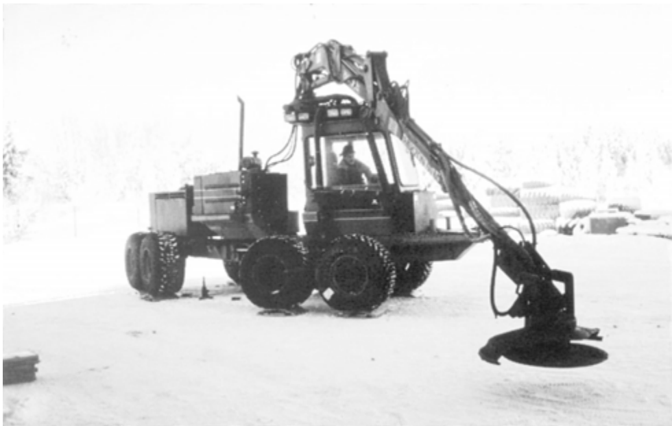
Fig. 1 The FMG Mini 678 cleaning machine, based on the original Bruunett Mini forwarder. The engine has been moved aft of the cab, and the knuckleboom loader has been mounted on the cab roof, making for excellent visibility. The machine has hydrostatic transmission, eight wheels, is 259-cm wide, has a ground clearance of 55 cm, weighs 11.4 tonnes and has a loader reach of 6.55 m.
