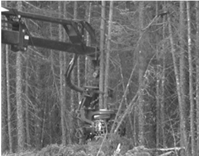
Figure 1. The accumulator arms that hold stems vertical after cutting.
