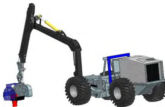
Figure 5. 3D rendering of a newly developed scarifier with soil inversion technique, here mounted on a modified Cranab FC8 forwarder crane and the off-road machine.
