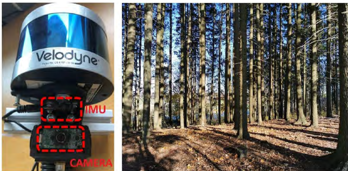
Figure 2. The handheld sensor platform used for data collection which consists of a lidar, an IMU and a camera. Data collection took place in a small forest.
