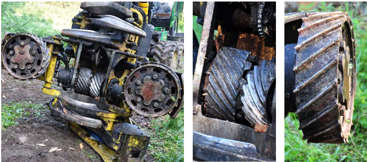
Figure 1. Adapted harvester head H415 with changed outer and inner feed rollers (left); inner feed rollers in detail (middle); outer feed roller in detail (right).
