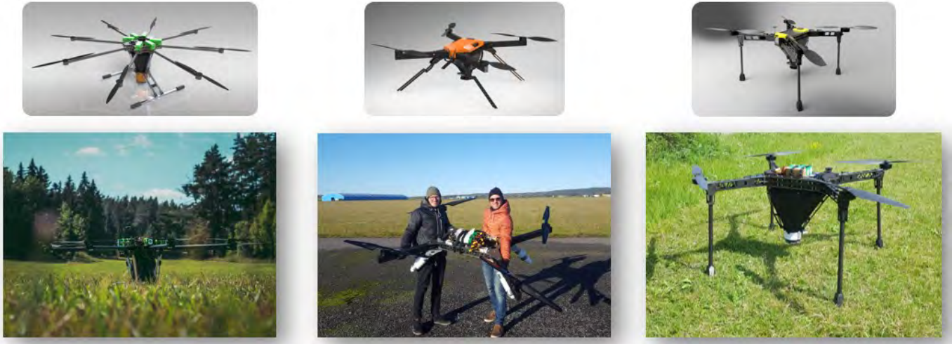
Figure 24. Drone development within Nordluft. From the left the first prototype BF 1, the second, BF 2 and to the right, the third prototype BF 2.1.
