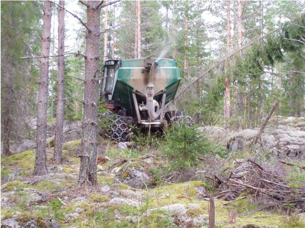
Fig. 19. A tractor spreading fertilizer in a conifer stand growing on mineral soil. Photo D. Malm
