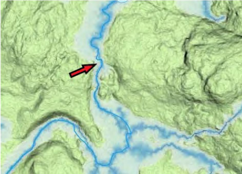
**Fig. 7. Finding suitable locations for stream crossings—Example 4** When a stream crossing is unavoidable, potentially suitable locations for placing a bridge can be identified on a wet area map in the office. Such locations are indicated where the blue zone adjacent to a stream is narrow. The suitability of the identified location can then be confirmed or revised by making a field inspection before the start of the operation.
