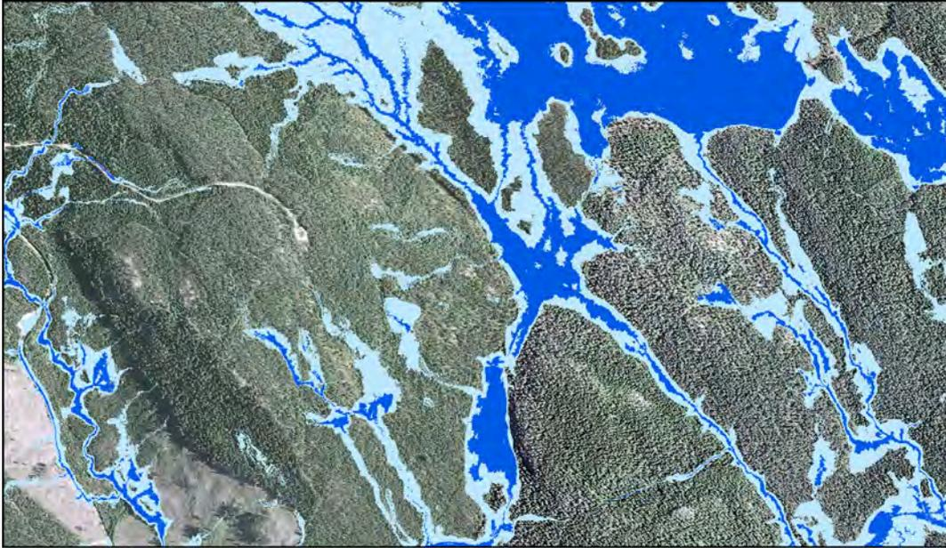
Fig. 28. This MLWAM shows three classes of soil moisture: dry-mesic (transparent, i.e. where the orthophoto is visible), mesic-moist (light blue) and moist-wet (dark blue).
