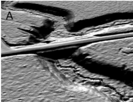
30A. In a 3D model of the land surface a road acts as an artificial dam.
