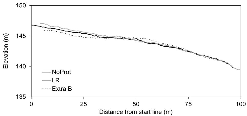
Fig. 7. Top: Size (in metres) of the study plots, and location of groundwater tubes (o) and transects T1-T6 at Trågalidsberget hillslope B. Bottom: Hillslope profiles of the study plots subjected to driving (note the different scales on the x- and y-axes, exaggerating inclination). The profiles show the interpolated original soil surface above the right rut, using GNSS-positioning and Triangular Irregular Networks. NoProt: No ground protection, LR: Logging residue, Extra B: Extra plot B.
