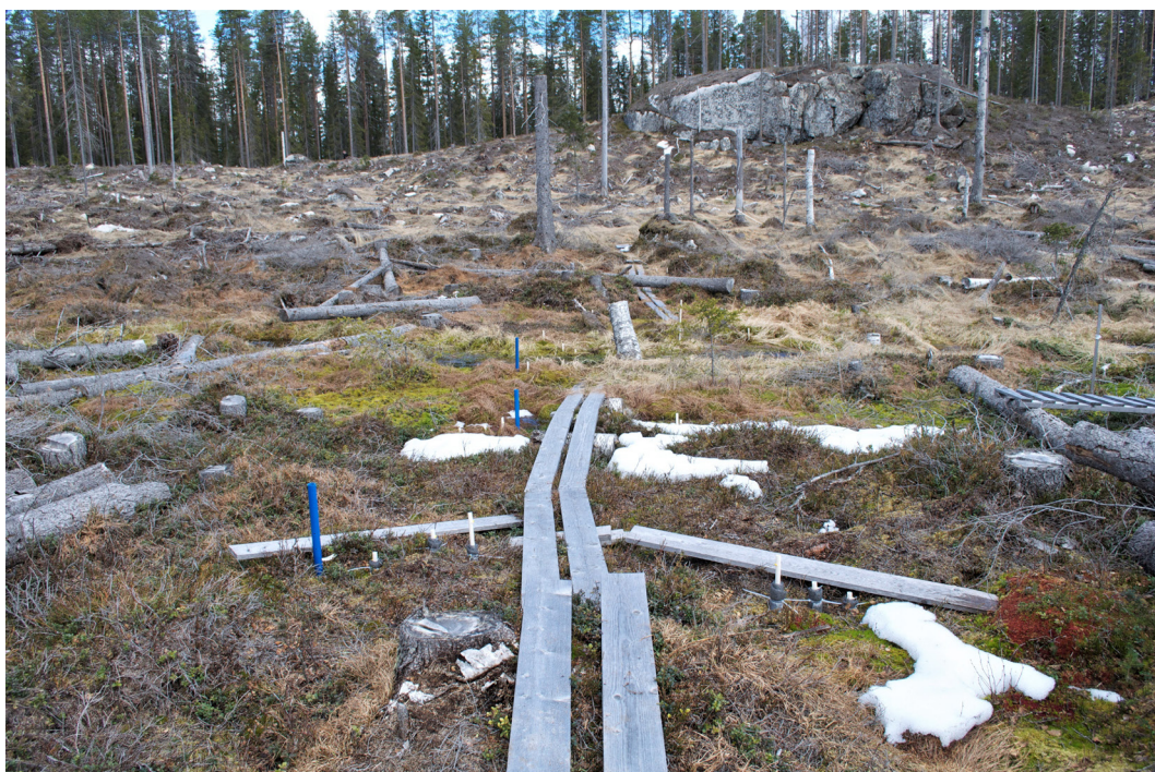
Figure 6. Piezometers and blue groundwater monitoring wells have been installed at four points (A-D) along two parallel lines on each side of the boardwalk. Here sampling positions A, B and C are shown. Photo E. Ring
