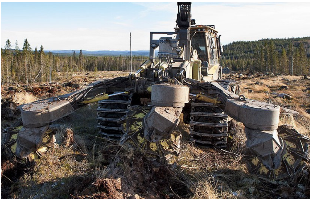
Figure 2. Scarification using 3-row disc trencher. A scarification is most often followed by a manual planting (photo: Lars-Göran Sundblad).
