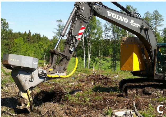
Figure 1. Some mounding-with-planting machines used in the Nordic countries.
