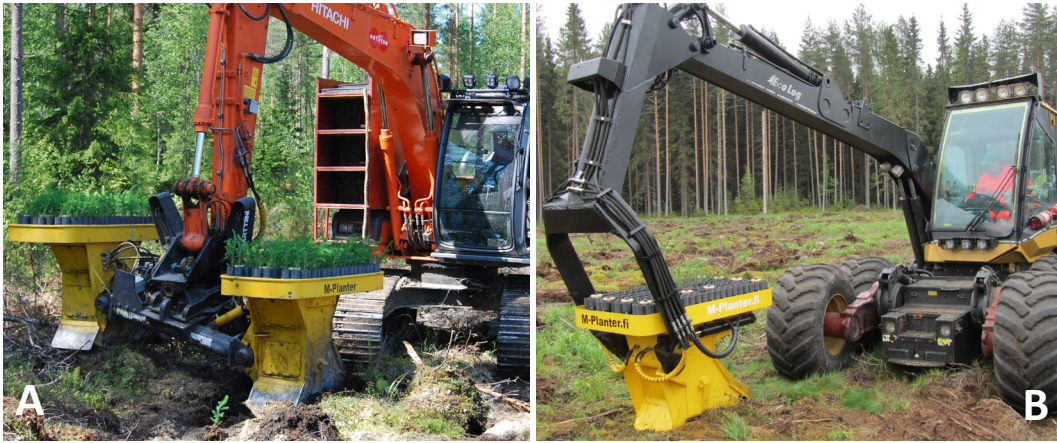
Figure 1. Some mounding-with-planting machines used in the Nordic countries.
