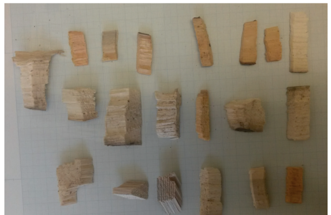
Figure 2. Examples of chips in the 16-32 mm class. Each large square = 10×10 mm, subdivisions 1 mm.
