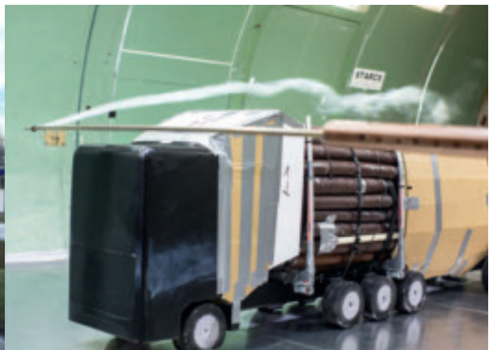
Fröjds Åkeri in Kisa owns one of the test trucks that was designed with a bigger cab deflector on the basis of the tests in the wind tunnel. It will also be fitted with a shield between the front wall and the first pair of stakes.
