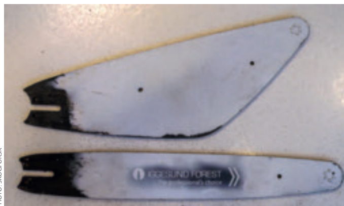
The new V-shaped saw bar and a conventional saw bar.
