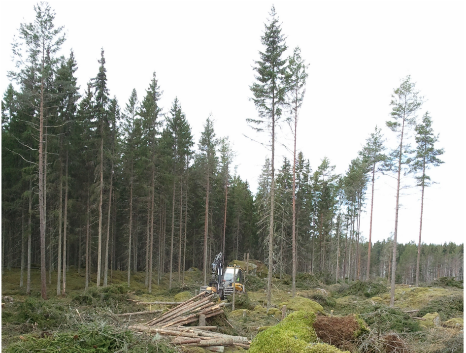
Figure 8. This harvester measures 64% of the diameters within \pm 4 mm from the manual control measurement. The standard deviation is 4.2 mm, while the systematic error is no less than -3.7 mm (left picture), indicating that the measurement system must be calibrated. By adjusting all diameter classes upwards by 3.7 mm, the harvester would, in theory, measure 76 % of the diameters within \pm 4 mm (right picture). If, in addition, you were to recalculate the entire base curve on the basis of the median in every diameter class, the harvester would, in theory, measure 79 % of the diameters within \pm 4 mm. Such a calibration would enable the harvester to measure very accurately.
