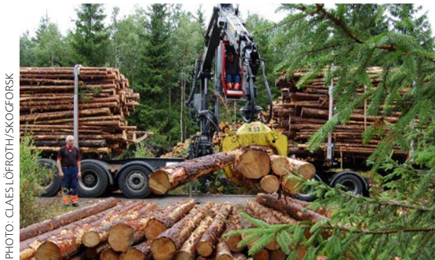
Figure 12. The Intermercato scale is mounted between the rotator and the boom tip. Instrument readings are placed in the crane cab.
