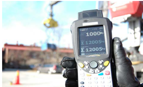
Figure 12. The Intermercato scale is mounted between the rotator and the boom tip. Instrument readings are placed in the crane cab.
