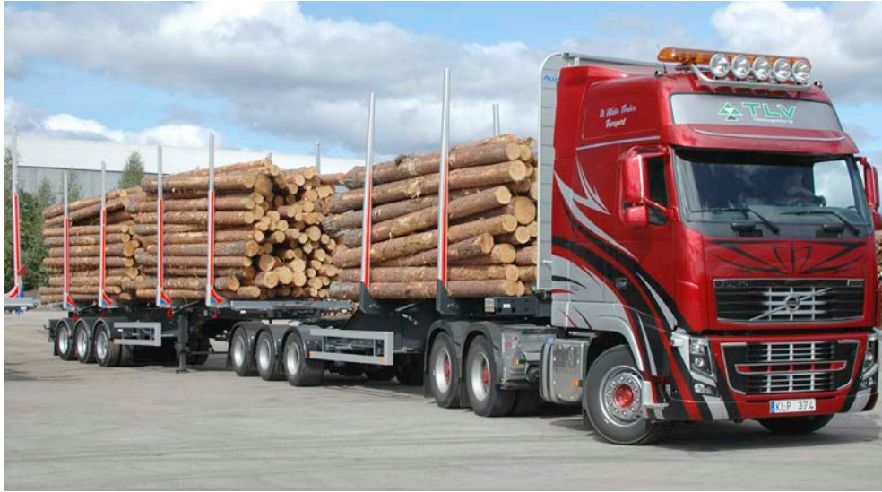
Figure 10. ST Tractor consist of a 6x4 tractor, a three axel link and a three axel trailer.
