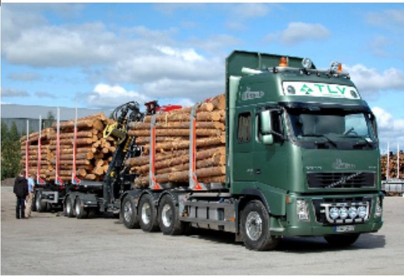
Figure 8. ST Crane consist of a 8x6 truck with crane, a two axel dolly and a three axel trailer.
