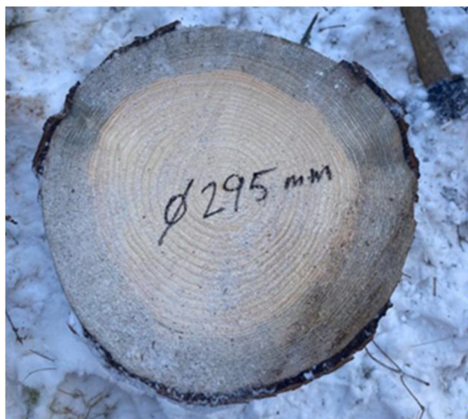
Fig E.1. Log with diameter 29.5 cm processed with frozen bark and with harvester head H415. Note feed roller tracks with ripped-off bark.
