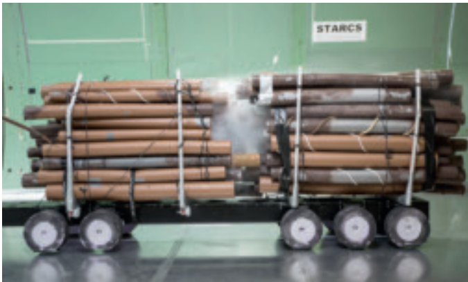
The wind flows through the timber load and forms eddies that slow the vehicle. The vehicle model is standing on a scale in the tunnel, where wind resistance is measured.
