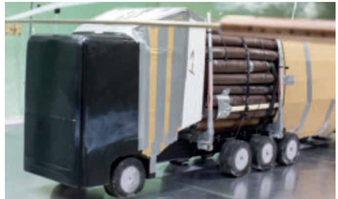
A prototype for the future. With this equipment, fuel consumption is reduced by 7-8 percent.
